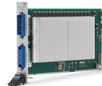
SLSC-12252 8-ch, 100V/30A FET FIU with Current Sense
