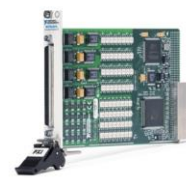
PXI-6515 \pm 30 VDC 32 Sink/Source Inputs, 32 Sink Outputs
