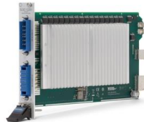
SLSC-12251 16-ch, 100V/8A FET FIU with Current Sense
